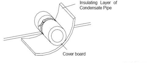
**Thermal Insulation of Condensate Pipe**
