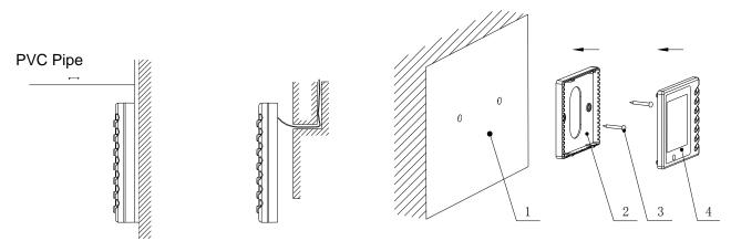
Fig 6 Surface Mounting of Cable
