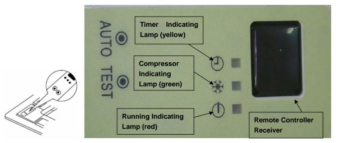
Instructions to the error indicating lamps on the dash receiver of the cassette type unit are described below. Once the handheld controller works, the error code will be displayed on it.
