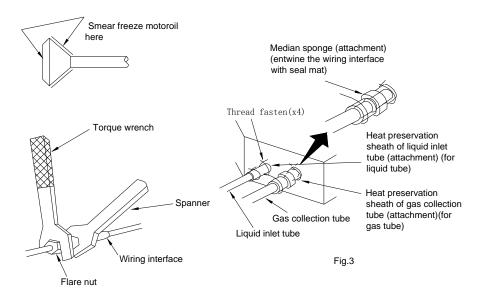
$\stackrel{<}{\succ}$  When connect the pipe to the unit or backout it from the unit, please do use both spanner and torque wrench. as shown in fig.3.
