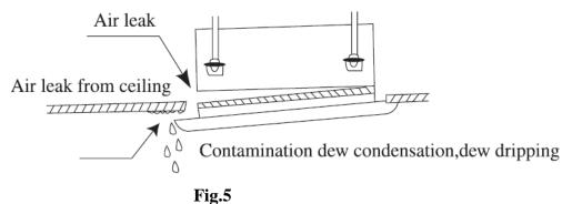
2. If gap is still left between the ceiling and the panel after screwing the screws, readjust the height of the indoor unit body (Refer to Fig.6)
