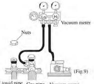
Liquid pipe Gas pipe Vacuum pump
