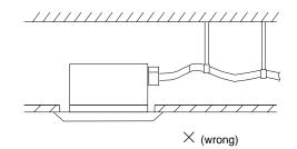
$\stackrel{}{\sim}$  Use the drain hose and clamp attached. Insert the drain hose to the drain vent, and then tighten the clamp.
